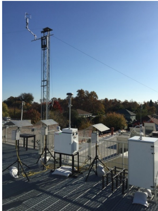
Figure 3. Three PM 2.5 sensors collocated with FRM and FEM instrumentation in Sacramento, CA, USA.
